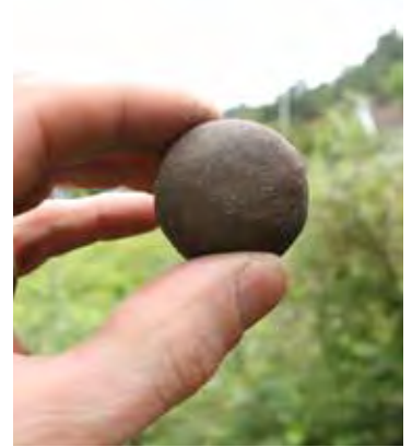
High Clay Content Soil Holds its shape and does not crumble when you poke it lightly.
