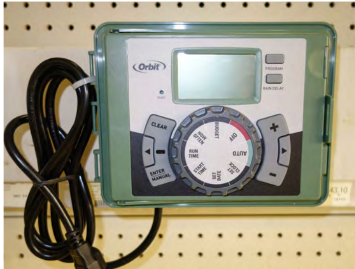
Figure 16. A programmable irrigation controller for multiple zones. More advanced units can become “smart” with the addition of soil moisture sensors and weather sensors.
