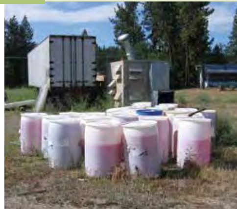
Chemical containers outside, without proper containment
